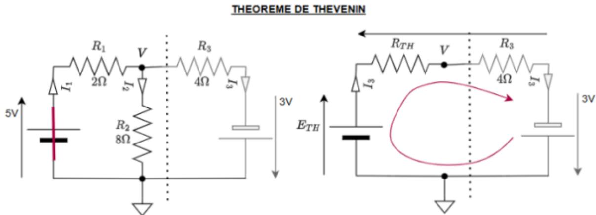
$$E_{TH} = \frac{R_2}{R_1 + R_2} \cdot 5 = 0.8 \cdot 5 = 4V$$
