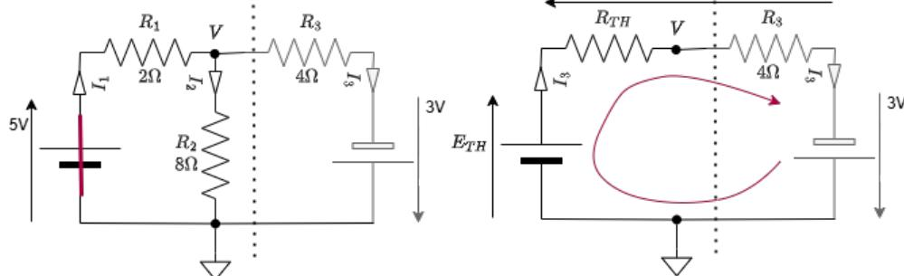
$$E_{TH} = \frac{R_2}{R_1 + R_2} \cdot 5 = 0.8 \cdot 5 = 4V$$
