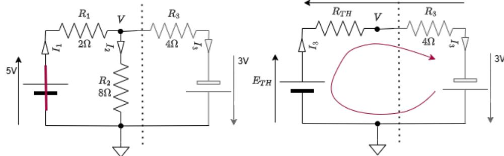
$$E_{TH} = \frac{R_2}{R_1 + R_2} \cdot 5 = 0.8 \cdot 5 = 4V$$
